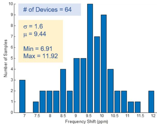
**Figure 5.1 Histogram of expected thermal cycle shift**
