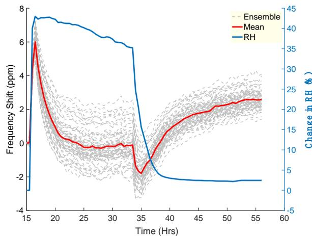
Figure 7.1 Frequency shift due to step changes in the RH profile in the temperature chamber
