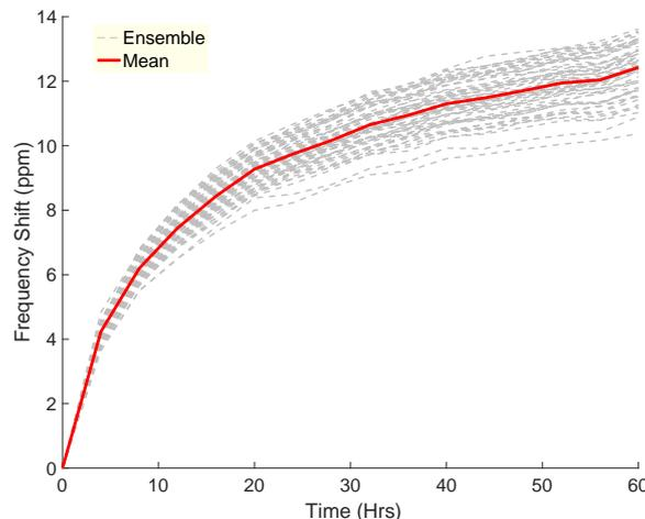
**Figure 9.1 Room temperature frequency shift over time after baking device at 100 °C.
