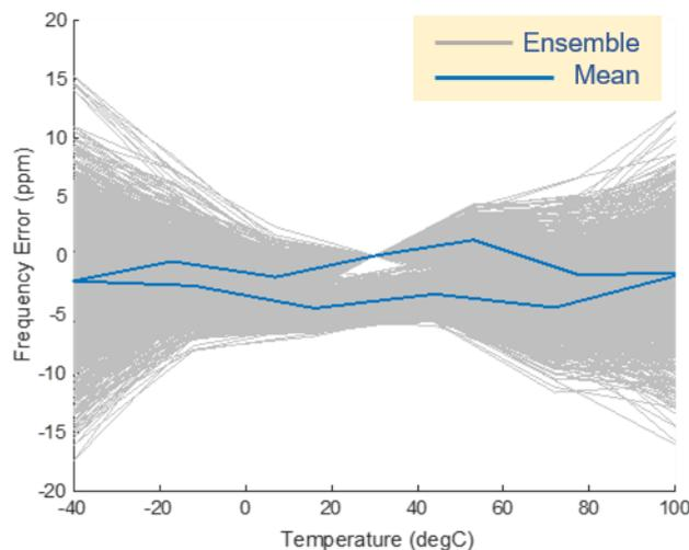
**Figure 5.2 Expected frequency error over temperature. Included are various process-corners**
