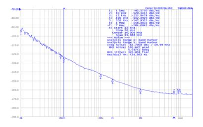
Figure 2.1. Phase Noise at 50 MHz
