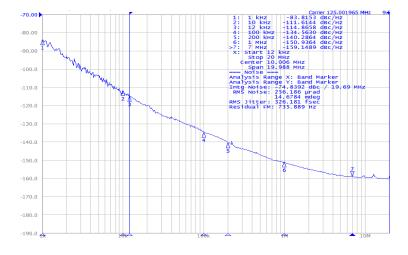
Figure 2.2. Phase Noise at 125 MHz
